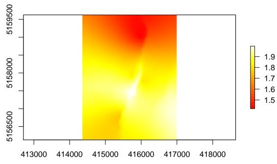
The image is a direct visualisation of potential locations of the seismic source. Usually, only values above the 95 (or 99) percentile are used to illustrate the location likelyhood. See the visualisation chapter from how to illustrate this trunctation and see the plot below for an example:
