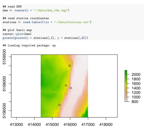
The Lauterbrunnen Valley is a steep limestone cliff with 600 m high, nearly vertical walls. Three seismic stations are located on top, one at the base of this impressive cliff. To create distance maps and interstation distances for this setting the following code is used (computation time for this 10 m DEM on one CPU more than one hour!):
